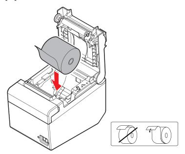
Pull out some paper, and close the roll paper cover. When the printer power is on, the roll paper is automatically cut. 3.
